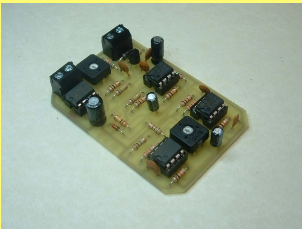
PICTURE 5: Fit screw terminal blocks & presets; plug in 4 x I/C chips last. NOTE! ANT-STATIC PRECAUTIONS REQUIRED
