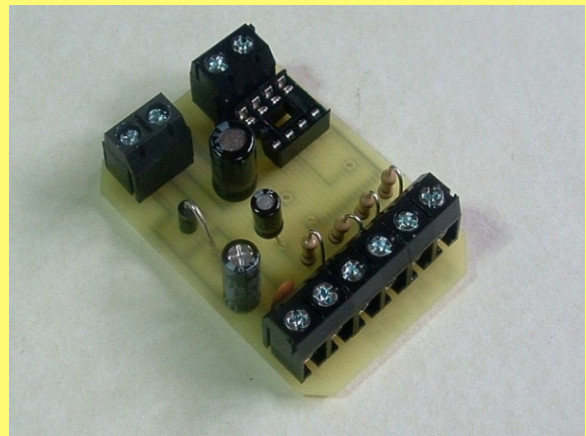
PICTURE 4: Capacitors fitted
