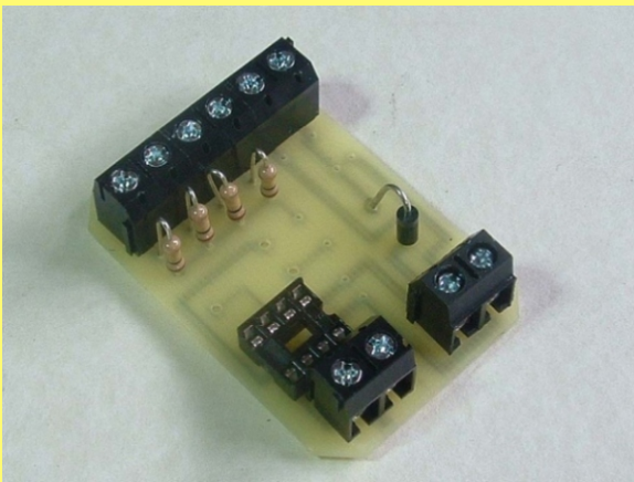
PICTURE 3: Resistors and diode fitted
