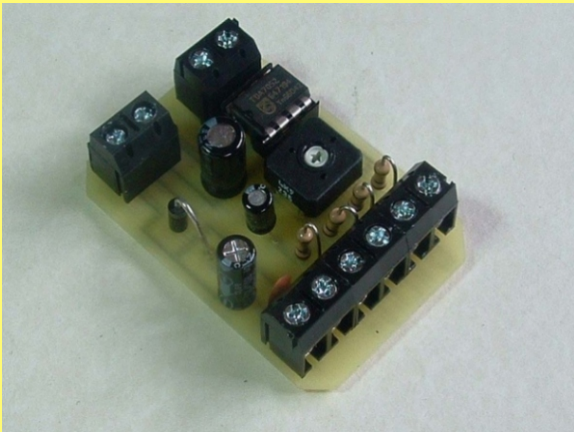
PICTURE 5: Preset and I/C chip added. ANTI-STATIC PRECAUTIONS REQUIRED!
