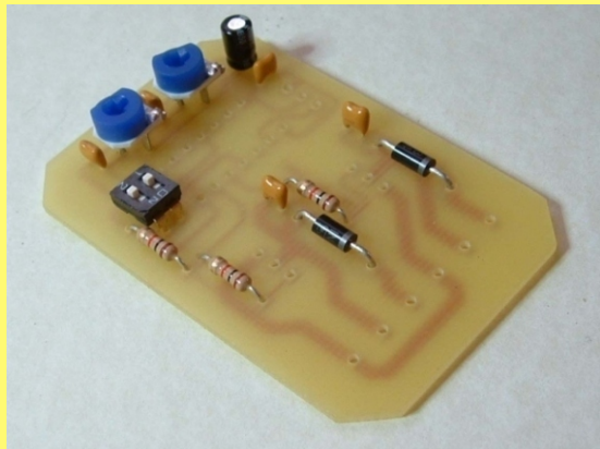
PICTURE 3: Trimmers and 2-way switches added
