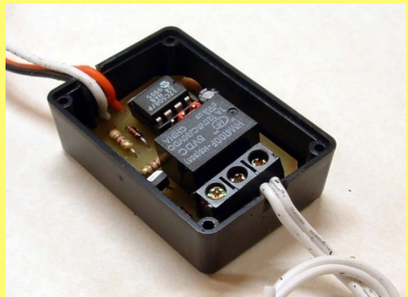
Picture 6 - Fit PIC chip; ANTI-STATIC PRECAUTIONS REQUIRED! File slots in case for cables
