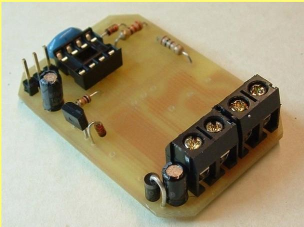
**PICTURE 3: Small MOSFET; remaining diodes, capacitors & terminal blocks fitted**
