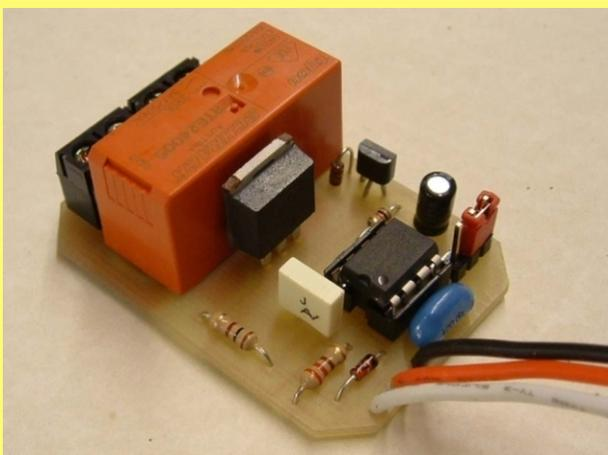
**PICTURE 5: Fit receiver lead and plug in PIC chip last.**
