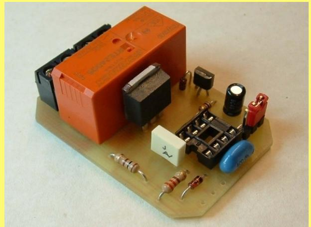
**PICTURE 4: Fit relay and main power MOSFET. NB! ANTI-STATIC PRECAUTIONS REQUIRED**
