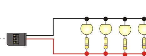
Spots - UltraBright LEDs with 470R series resistors
