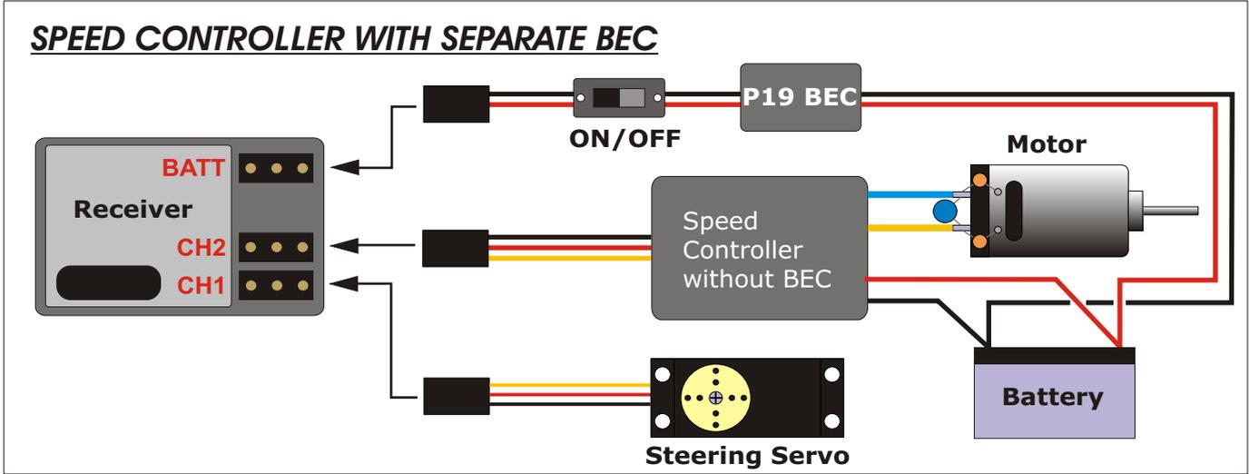
A separate BEC is not as convenient as one built into the ESC, but I feel that technically it is a better solution - it allows you more flexibility in the way you segregate power".
