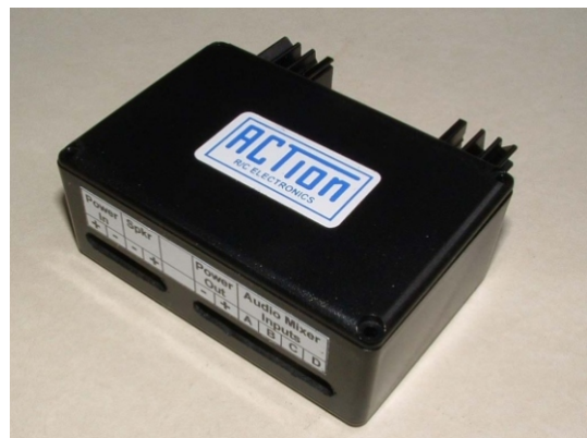
Picture 8: Shows finished unit in case with self-adhesive logo and connections legend.
