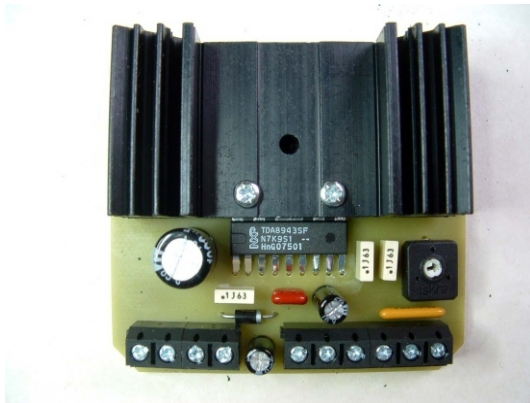
Picture 5: Shows all other PCB components soldered in place.
