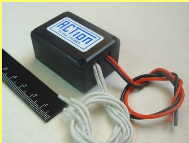
PICTURE 5: File slots in case for leads. Fit lid and sticker
