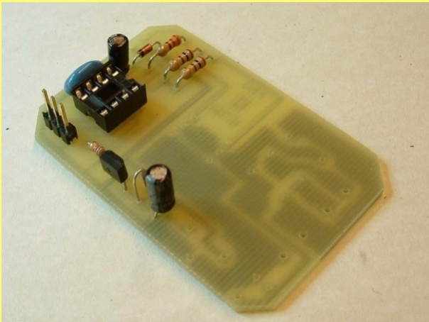
PICTURE 3: Small MOSFET; further diode and capacitor fitted
