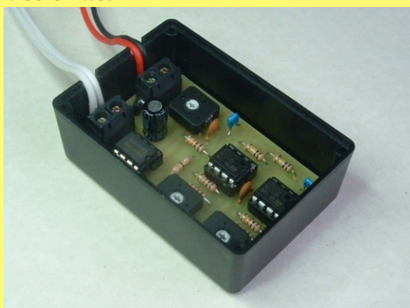
PICTURE 6: File slots in case for cables
