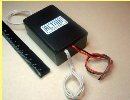
PICTURE 7: File slots in case for leads; fit lid and sticker. White leads at front are motor connections; speaker leads at rear.
