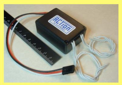
PICTURE 5: Finished unit, cased with sticker. Each pair of white wires is COM and NO for one of the relays.
