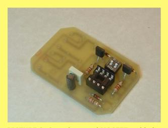
**PICTURE 3: Capacitors and MOSFETs added**
