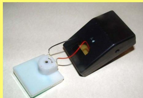
**8. Assemble case and fit meter**
