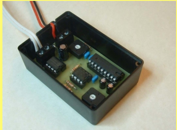
PICTURE 6: File slots in case for cables
